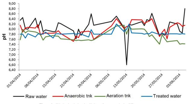
Figure 4. pH behavior during the 60 days of treatment in the different stages
