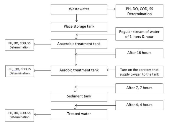
Figure 2. Operational flow diagram of the proposed prototype. The acronyms of DO refer to dissolved Oxygen, Chemical Oxygen Demand (COD) and SS suspended solids.
