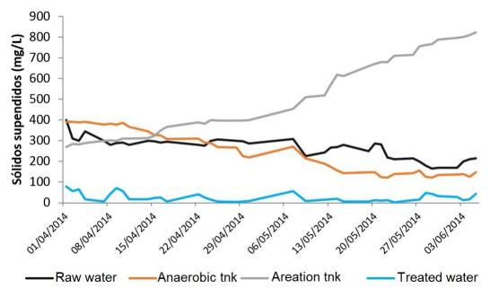
Figure 6. Behavior of total suspended solids during the 60 days of treatment in the different stages
