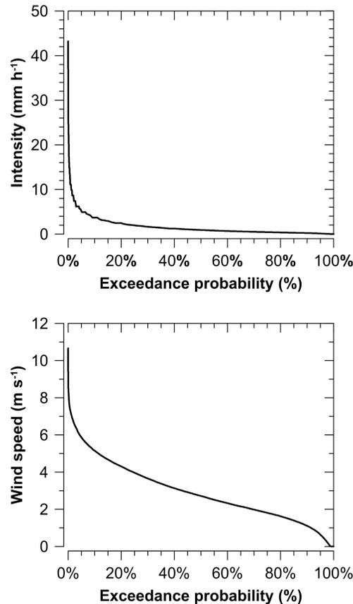
**Figure 2.** Rainfall intensity exceedance probability curve of the 5-min rainfall data collected by the TE525MM gauge (**top**), and wind speed exceedance probability curve of the corresponding 5-min intervals (**bottom**).
