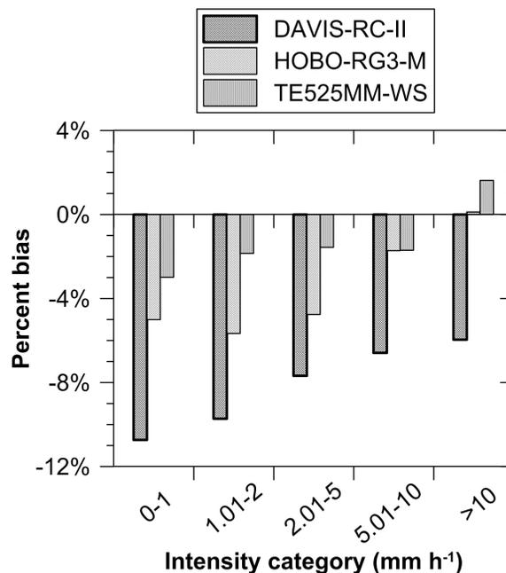
**Figure 4.** Percent bias of the Tipping-Bucket (TB) rain gauges in relation to the TE525MM sensor as a function of rainfall intensity. The data used for this figure corresponds to the highlighted categories in Table 3.
