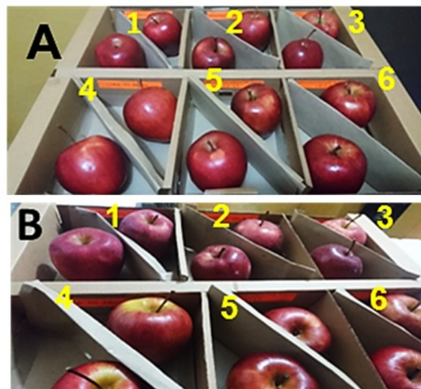
Figure 6. A. Preservative boxes with apples at the beginning of the test and B. Preservative box at 30 days (1 control, 2 Ag-NPs at 5:5, 3 Ag-NPs at 5:10, 4 bee wax, 5 bee wax and Ag-NPs at 5:5 and 6 bee wax and Ag-NPs at 5:10)
