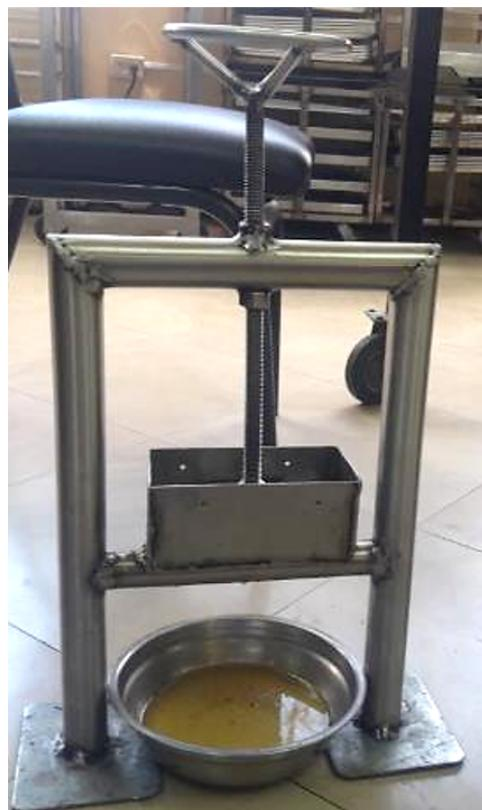
**Figure 1.** Manual press oil extractor
