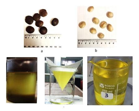
Figure 1. a) SI seed with shell. b) SI seed without shell. c) Product obtained after the extrusion. d) Oil filtration. d) Filtered oil.
