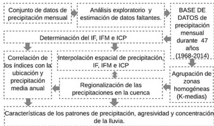
Figure 2. Methodological scheme for the regionalization, aggressiveness and concentration of the rain time series.
